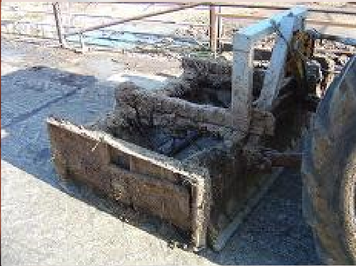
Fig 3: A box scraper will scrape cleanly, especially along kerbs, but will also save labour time making it an extremely cost effective investment
